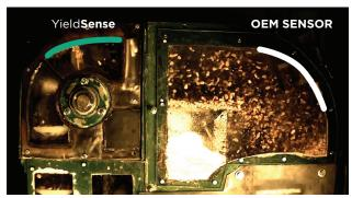
Showing low grain flow across sensor areas. Much of the grain doesn't even hit the other yield sensors (shown in white).
